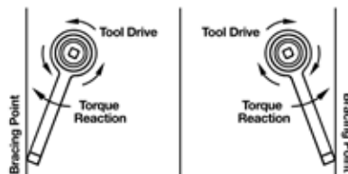
Torque Bar Opposes Rotation of Tool
